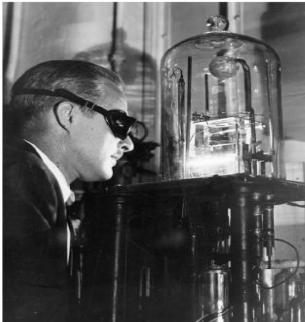
Walter Houser Brattain (1902–1987), experimenting with metal contacts on copper oxide (1935) at Bell Telephone Labs. A vacuum evaporation chamber is used to deposit the metal electrode.
