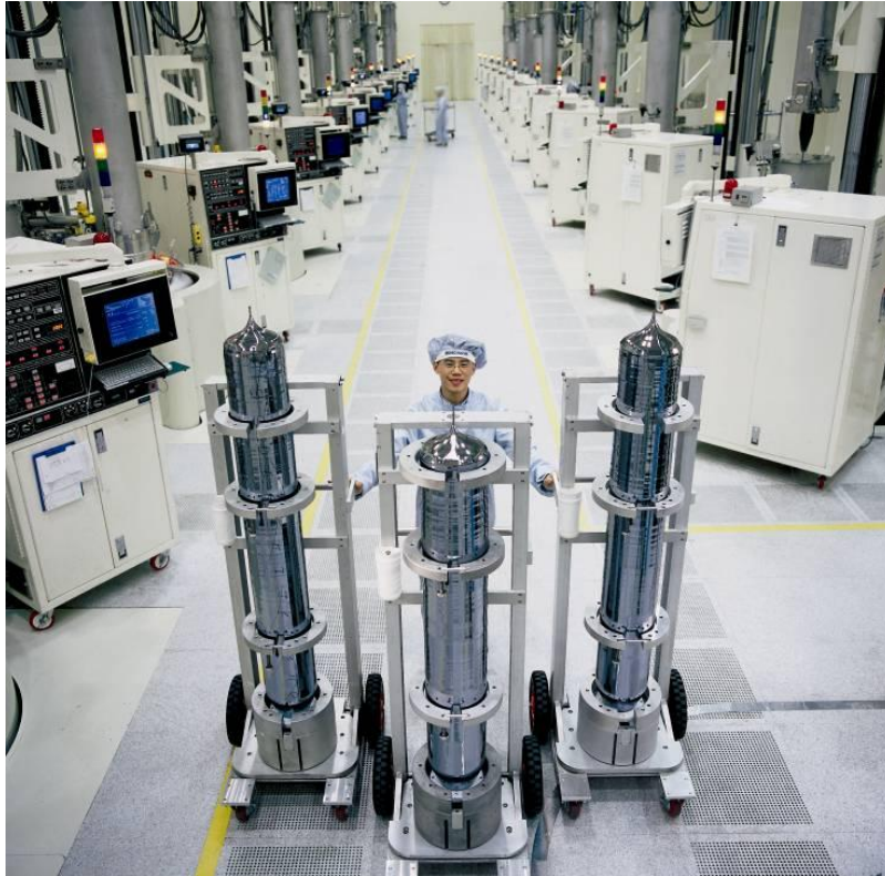
Left: Silicon crystal ingots grown by the Czochralski crystal drawers in the background
